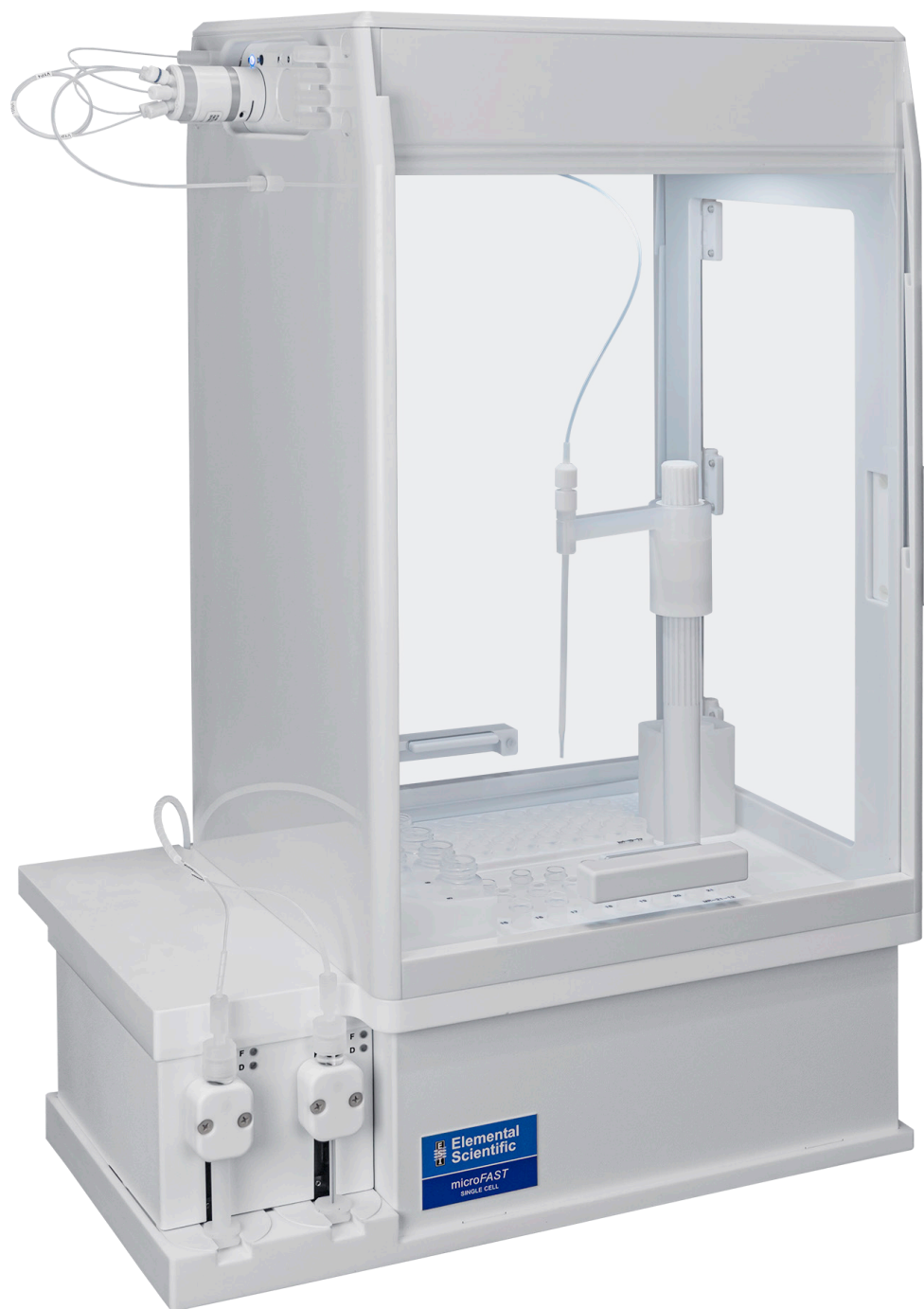
microFAST Single Cell Automated Sample Introduction System
